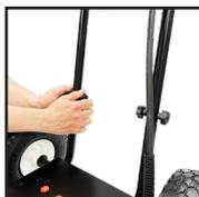
3. Attach the Cart Top/Reel to the Cart Base. A rubber mallet may be helpful to fully insert. Hand-tighten the star bolts to secure.
