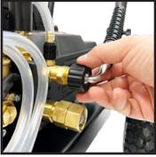
4. Attach the 22" black jumper hose to the outlet of the unloader. Hand tighten until secure.
