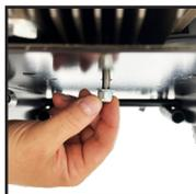
2. Once placed on the Cart Base, remove protective rubber caps from mounting studs. Using 13mm wrench, secure the Pump Unit using the 4 washers and 4 nuts (included).
